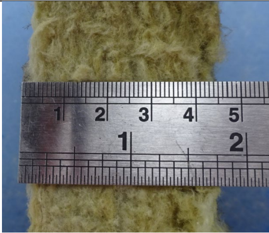
Figure 43: General view to confirm thickness of mineral wool insulation batt – 45mm.
