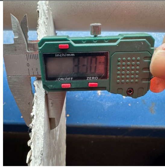
Figure 40: General view to confirm thickness of Steni GRP rainscreen cladding panel – 8mm.
