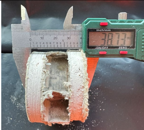
Figure 33: General view to confirm thickness of the Paramount partition lining board – 38mm.
