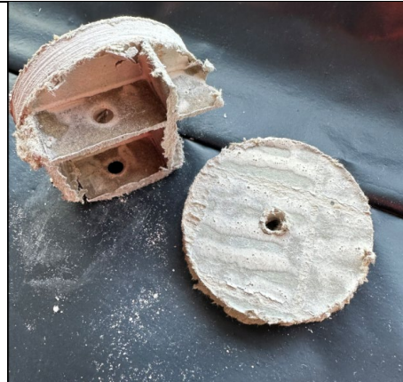
Figure 32: Alternative view of Paramount partition lining board which comprises of two layers of 10mm plasterboard with an 18mm honeycomb cardboard core.
