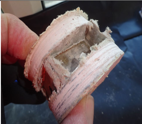
Figure 31: Alternative view of Paramount partition lining board which comprises of two layers of 10mm plasterboard with an 18mm honeycomb cardboard core.
