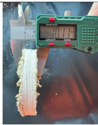
Figure 52: General view to confirm thickness of the plasterboard – 10mm.
