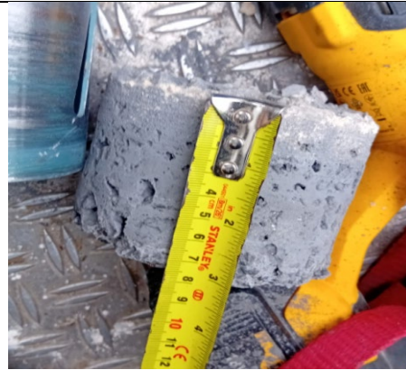
Figure 36: General view of core sample to show 60mm blockwork with 20mm pebble dash render finish.
