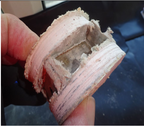
Figure 49: Alternative view of Paramount partition lining board which comprises of two layers of 10mm plasterboard with an 18mm honeycomb cardboard core.
