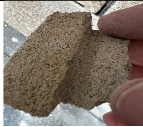
Figure 64: General view of a section of the blockwork inner leaf.
