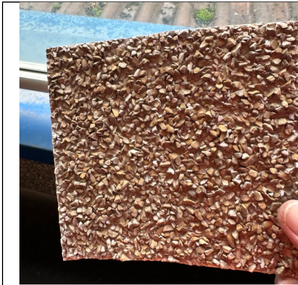
Figure 57: General view of Steni GRP rainscreen cladding panel.
