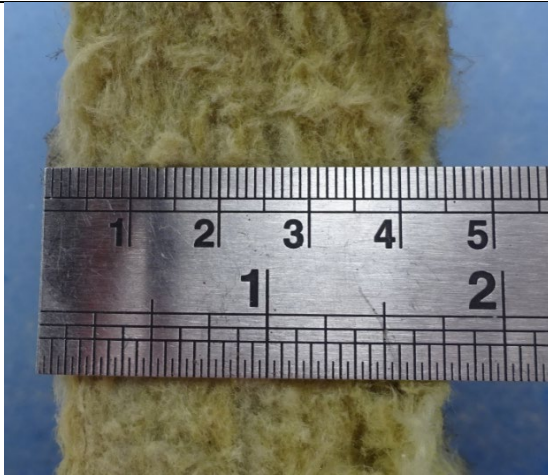
Figure 61: General view to confirm thickness of mineral wool insulation batt – 45mm.
