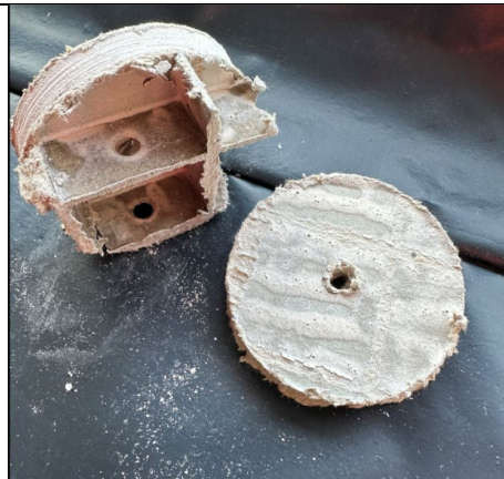
Figure 50: Alternative view of Paramount partition lining board which comprises of two layers of 10mm plasterboard with an 18mm honeycomb cardboard core.
