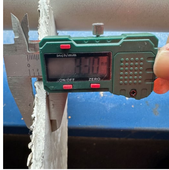
Figure 58: General view to confirm thickness of Steni GRP rainscreen cladding panel – 8mm.
