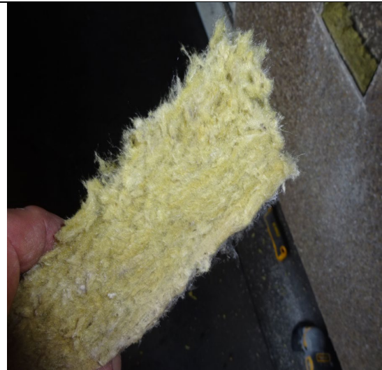
Figure 60: General view to show mineral wool insulation batt.
