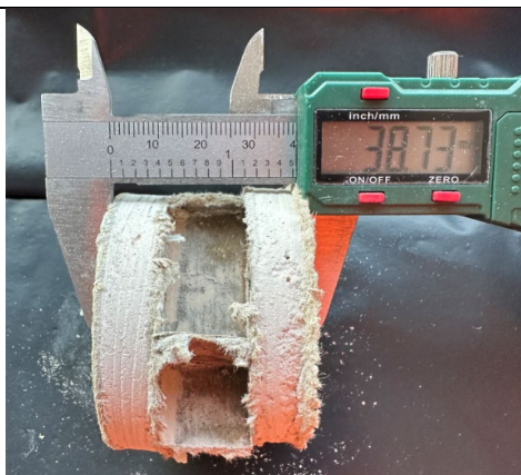
Figure 51: General view to confirm thickness of the Paramount partition lining board – 38mm.
