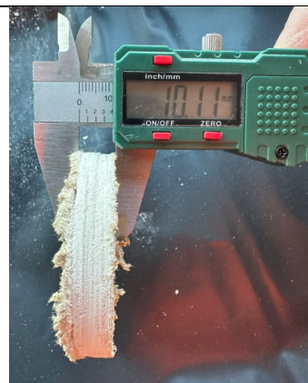
Figure 52: General view to confirm thickness of the plasterboard – 10mm.
