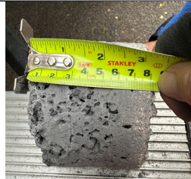
Figure 36: General view of core sample to show 60mm blockwork with 20mm pebble dash render finish.
